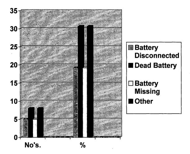
The fire fighters found 26 smoke alarms that failed when testing during the smoke alarm survey process. Dead batteries were a major cause in 8 or 30.7% of the non-functioning smoke alarms. Missing batteries was the cause in 5 smoke alarms or 19.2% along with another 5 or 19.2% with the battery disconnected; 8 other smoke alarms failed for one reason or another, possibly because of the age of the detector.
